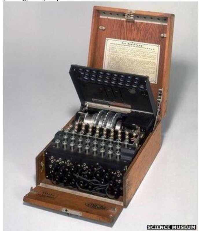
Gambar 2.8 Mesin cipher enigma
